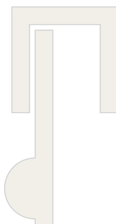
Channel Section attached to grille (side view)
