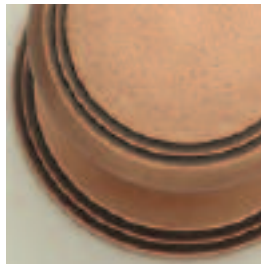
weathered copper (WC)
